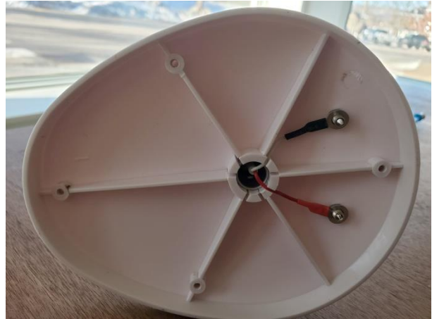
Step 4 - Place the wires on their respective terminals and replace the nuts. Before the base is reassembled and to make sure the wires are not crushed by the metal plate, push the wires into the slots provided.
